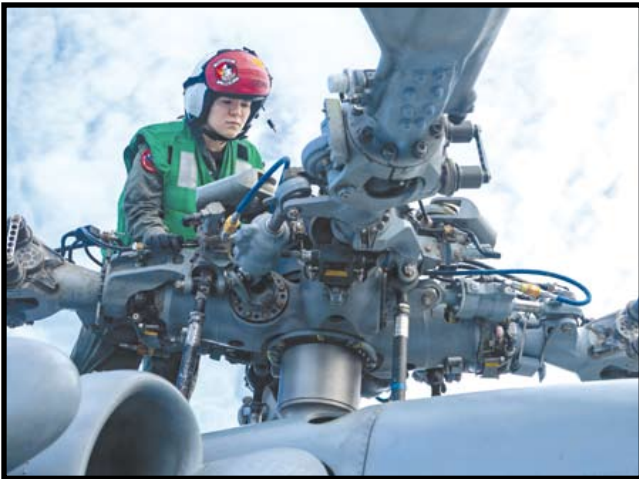
PREFLIGHT CHECK Navy Lt. Danaikiss Betancourt inspects the main rotor of an MH-60R Sea Hawk helicopter during a preflight check aboard USS Rafael Peralta in the Philippine Sea, Jan. 8, 2026. U.S. Navy photo by Petty Officer 1st Class Ryre Arciaga
